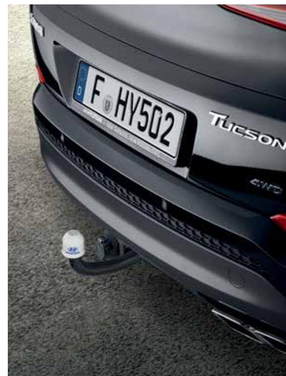
Tow bar, fixed. Ideal for regular use, this fixed tow bar features a high-quality corrosion-resistant coating. Certified according UNECE to 55R. Consult your dealer for the maximum payload of the bike carrier usage. D7280ADE00
