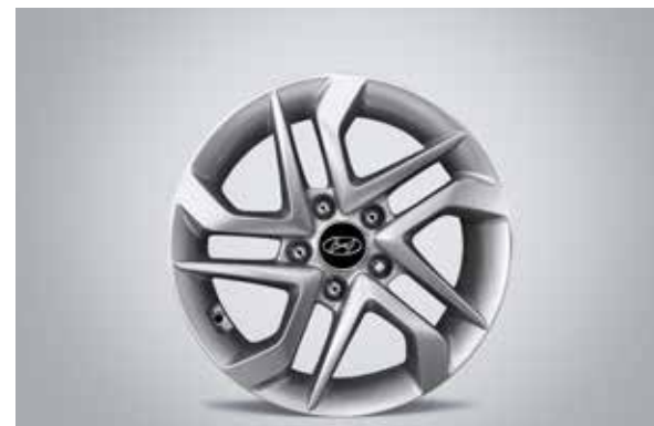
1. Alloy wheel 16". 16" five-double-spoke alloy wheel, 6.5Jx16, suitable for 215/70 R16 tyres. Not for vehicles with electric parking brake. Cap and nuts not included. 52910D7110PAC
