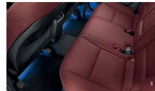
1.-4. LED lighting foot area. Concealed floor illumination for the front and rear foot space. It provides welcome illumination that automatically switches on and off with the opening and closing of the front doors. Upon starting the engine the illumination dims out. Available in blue and white coloured illumination. 99650ADE00W (White, 1st row) / 99650ADE10W (White, 2nd row) / 99650ADE00 (Blue, 1st row) / 99650ADE10 (Blue, 2nd row) 2nd row only in combination with 1st row LED lighting.
