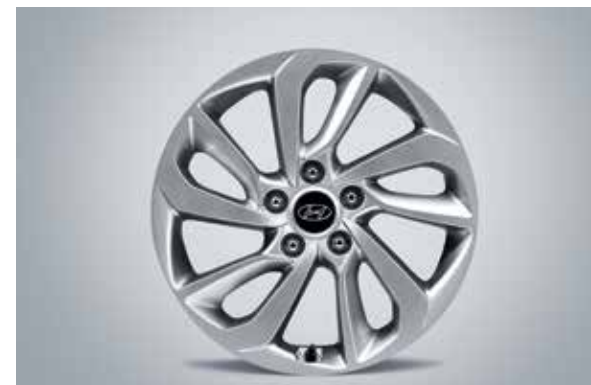
2. Alloy wheel 17". 17" ten-spoke alloy wheel, silver, 7.0Jx17, suitable for 225/60 R17 tyres. Cap and nuts not included. 52910D7210PAC
