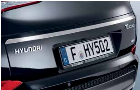
Tailgate trim line. Created to complement other design details, this high gloss stainless steel strip brings a stylish finishing touch to the tailgate. D7491ADE00ST
