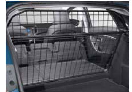
Cargo separator, above and below. The ideal solution to keep the boot area separate from the passenger area when the back seats are folded down. A6151ADE00 (below)
